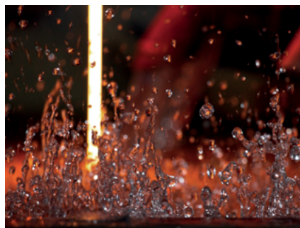
Frit is melted at 1450 °C
