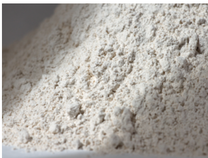
Feldspar, the main component or frit production
