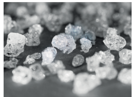
Produced glass-like granules are used to make glaze
