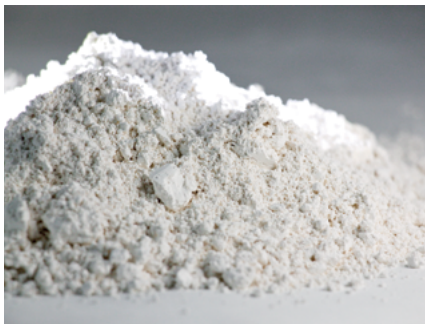
Zirconium silicate gives glaze its white colour
